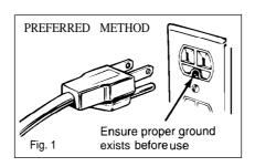
**WARNING-improper**use of the grounding plug can result in a risk of electric shock.
